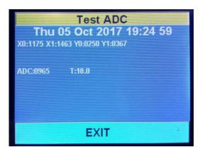
Here are shown the two calibration points(X0, Y0) and (X1, Y1) The instant value of the ADC and the corresponding Calculate temperature. X0 is the ADC value of the cold point, X1 is the ADC value of the hot point. Y0 is the temperature of the cold point, Y1 is the temperature of the hot point.
